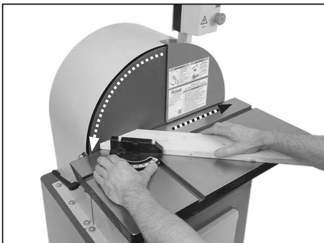
Figure 12. Example of angle sanding.
